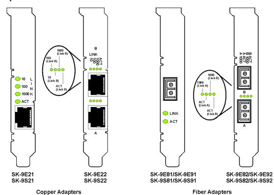
Figure 4. Location of the LEDs (adapter variant 1)
